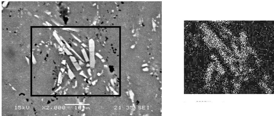
**Figure 4.** Dot mapping of intermetallic phases in AA5754.
