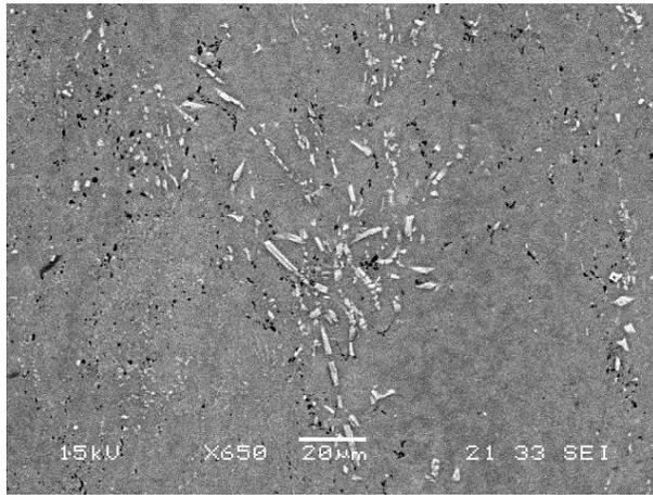
**Figure 1.** Surface segregations on the as-cast AA5754.
