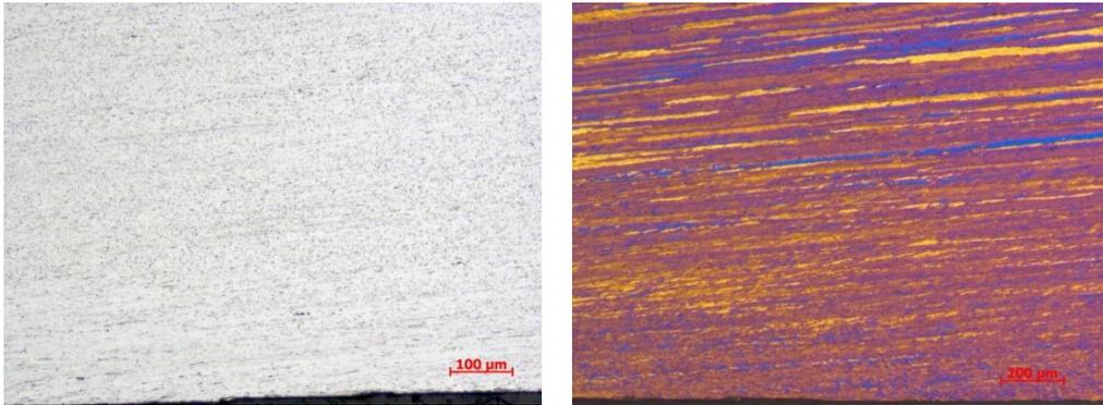
Figure 1. Microstructure of as cast TRC AA1050.
