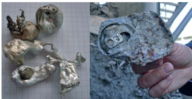
Molten aluminium and cans recovered from bottom ash (picture courtesy of EAA)
